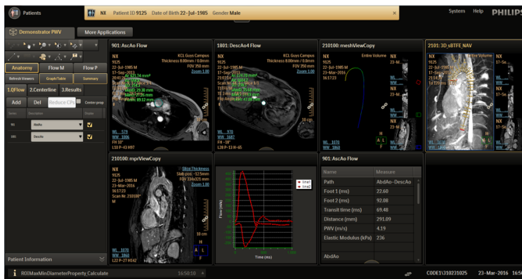
Fig. 4. Screenshot of the software. The left pane shows the tabs for the different steps to guide the user. The right pane shows on top from left to right the two PC MRI images with the aorta segmented, a color-coded centreline displaying area, the segmented artery, and on the bottom row the MR image used to define supra-aortic end points, input flow curves and table with results.
