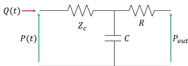
$$P(t) = Z_c Q(t) + \frac{1}{C} e^{-\frac{t}{RC}} \int_0^t e^{\frac{t'}{RC}} Q(t') dt + (DBP - P_{out}) e^{-\frac{t}{RC}} + P_{out}$$
